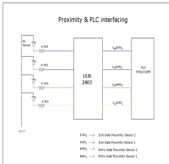
Fig. 2: Wiring diagram for PLC and Sensor interface
