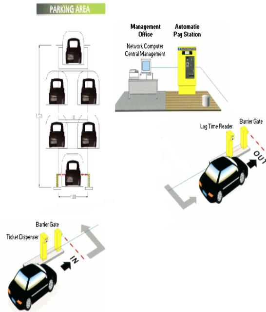
Fig. 4: Schematic view of overall parking system
